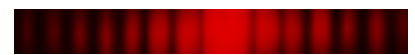
w / Single-slit diffraction of red light. Note the double width of the central maximum.
